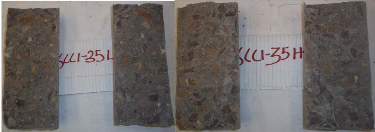
Figure 4.9 Coarse Aggregate Distribution for SCC1-35
