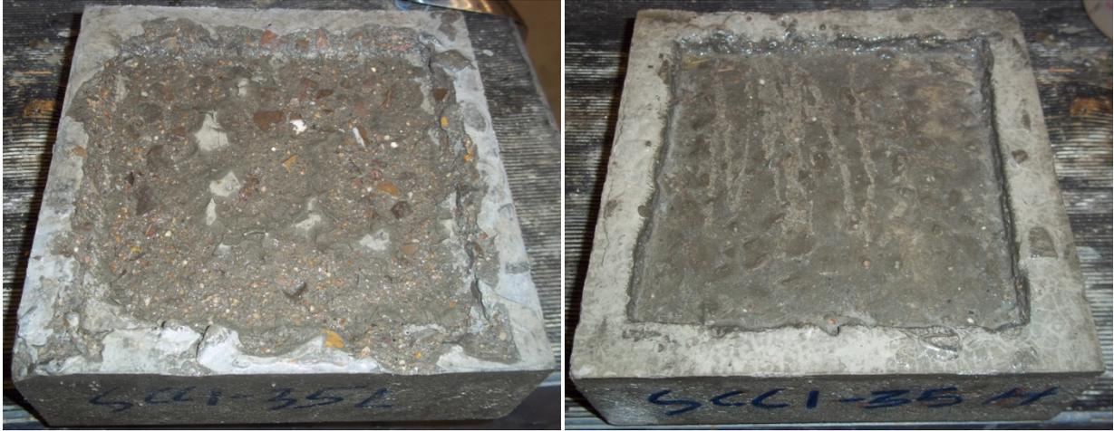
Figure 5.15 SCC1-35L (Left) and SCC1-35H (Right) after 15 freezing and thawing cycles
