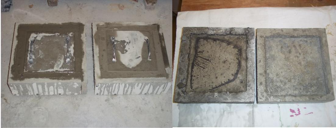
Figure 4.13. Fabrication of Specimen Molds for Surface Scaling Test
