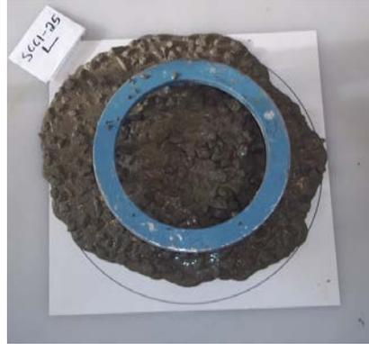
Figure 4.2 J-Ring Flow Diameter for SCC1-25L
