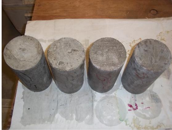
Figure 5.9 Fabricated Specimen after 1 week Immersion Period
