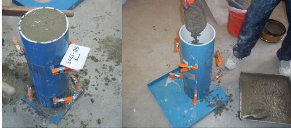
Figure 4.3 Static Column Segregation Test Setup for SCC1-25L
