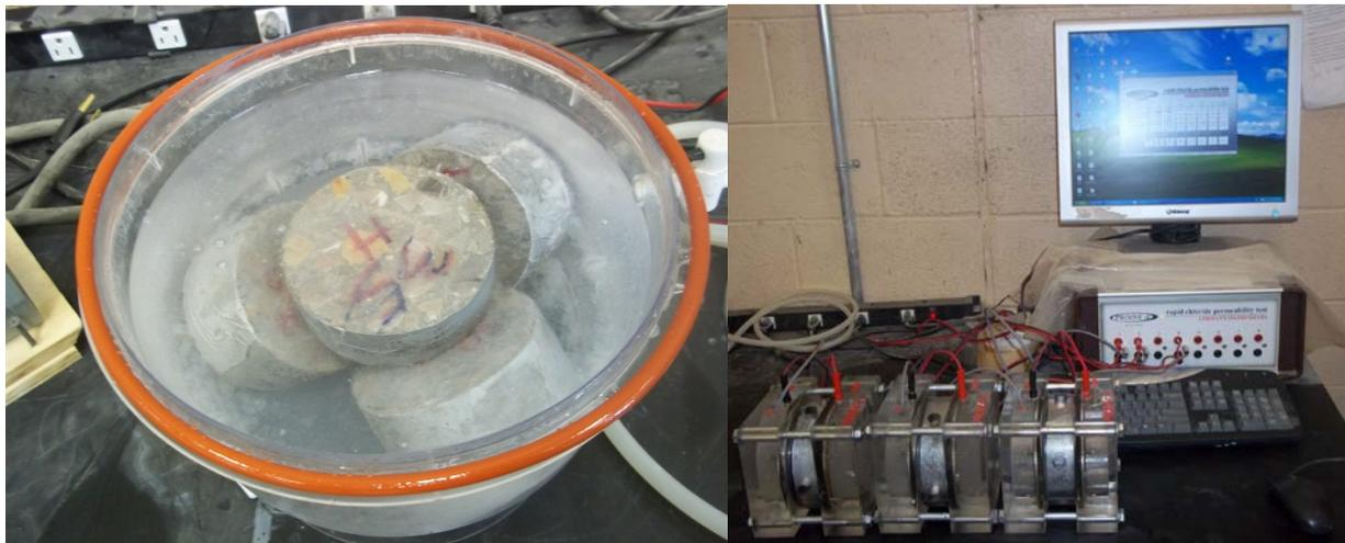
Figure 4.11 Experimental Setup for RCPT
