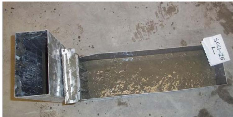
Figure 4.4 L-Box Experimental Setup for SCC1-25L
