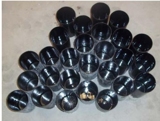
Figure 4.5 Lubricated Cylindrical Molds for Specimen Fabrication
