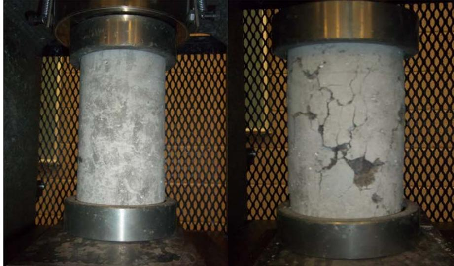
Figure 4.6 Experimental Setup for Compressive Strength Testing
