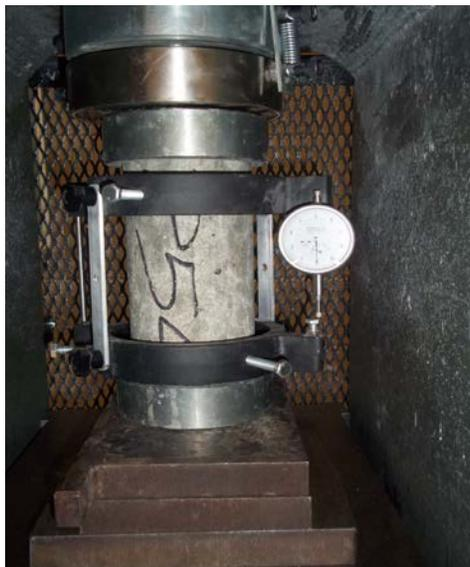
Figure 4.10 Experimental Setup for Static Modulus of Elasticity Testing
