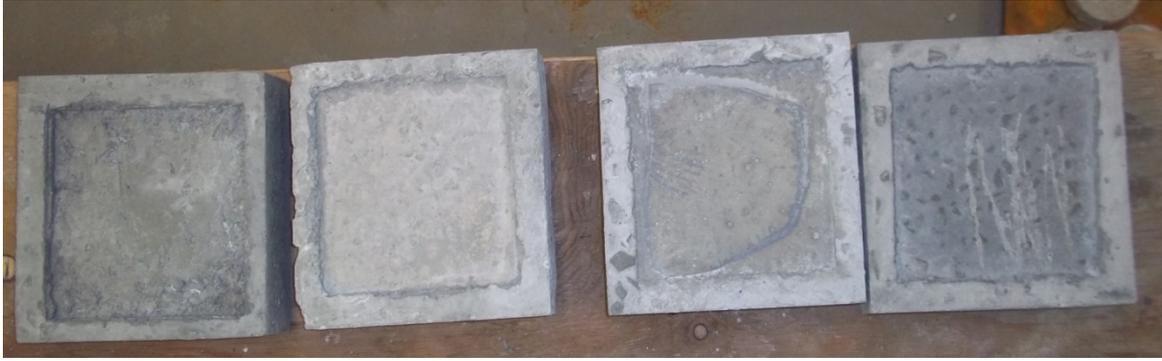
Figure 5.10 Specimens prior to commencement of freezing and thawing cycles
