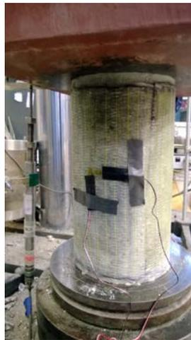
Figure 6.3: Test setup and instrumentations
