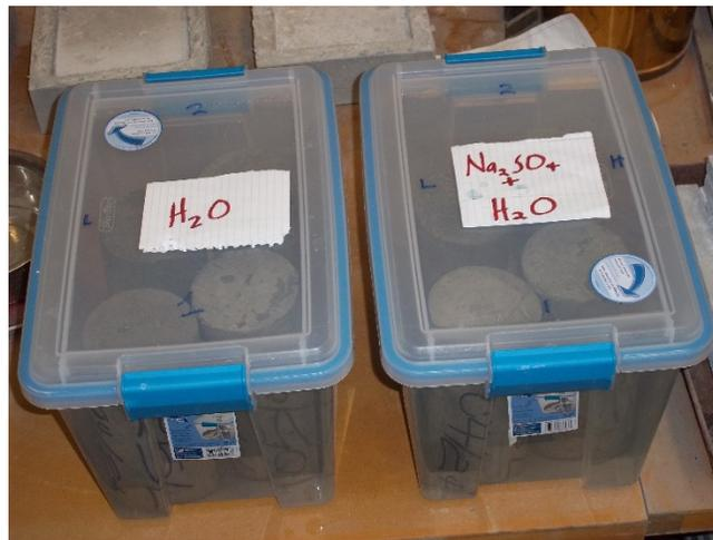
Figure 4.12 Sulfate Attack Experimental Setup
