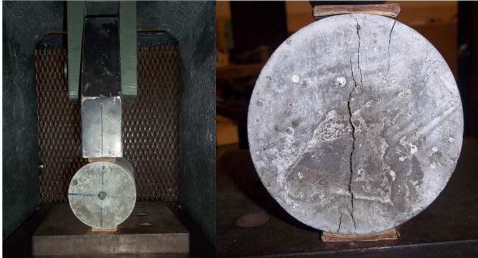
Figure 4.7 Experimental Setup for Splitting Tensile Strength
