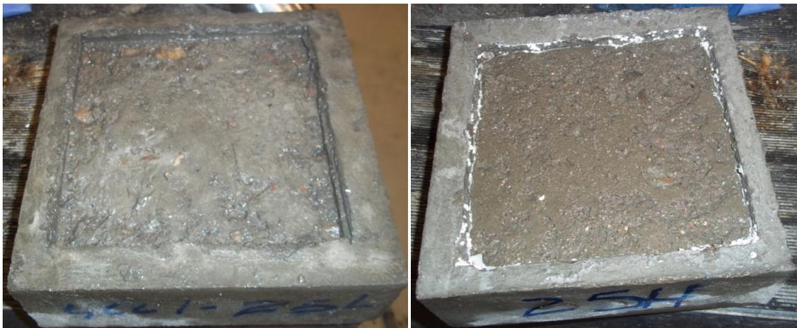
Figure 5.14 SCC1-25L (Left) and SCC1-25H (Right) after 15 freezing and thawing cycles
