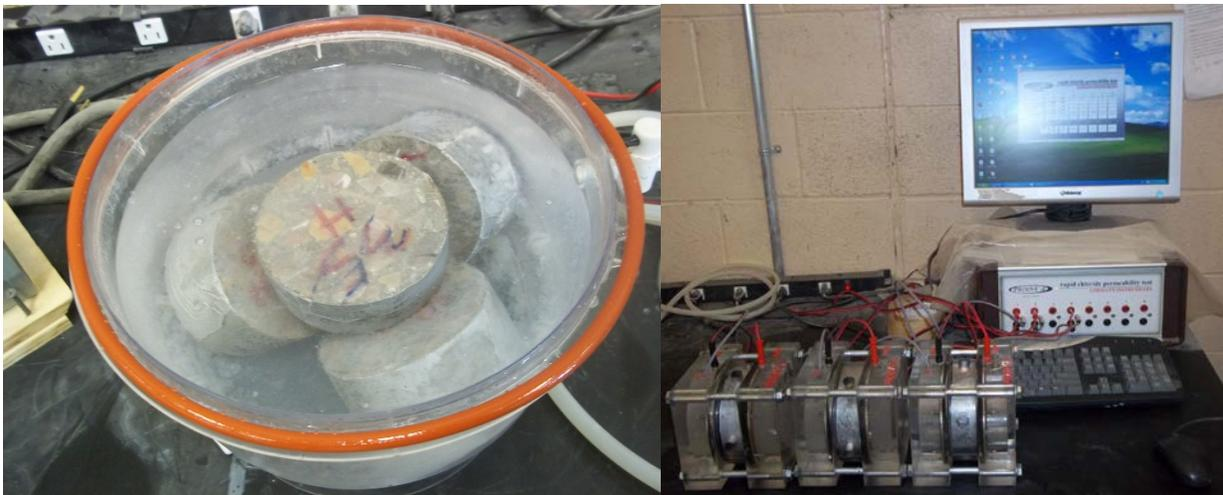
Figure 4.11 Experimental Setup for RCPT
