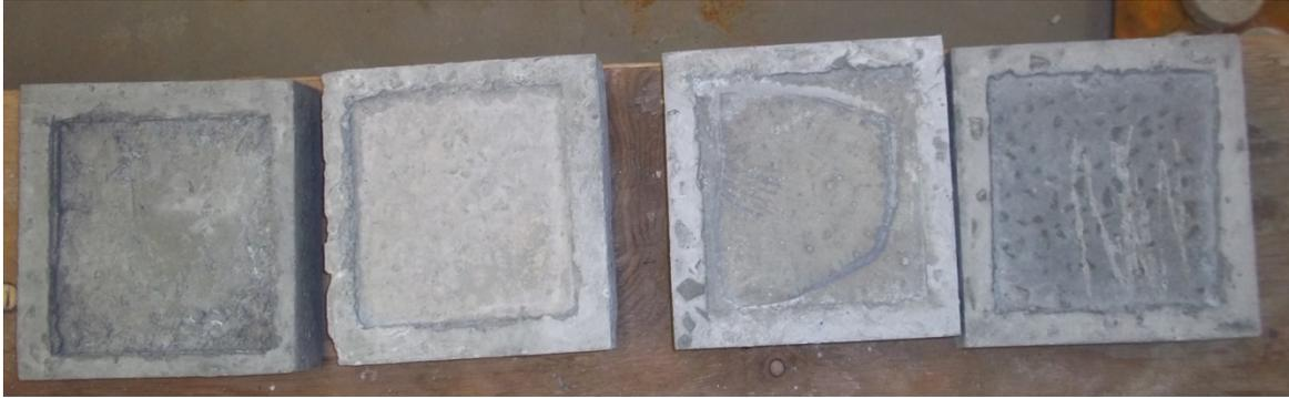
Figure 5.13 Specimens prior to commencement of freezing and thawing cycles
