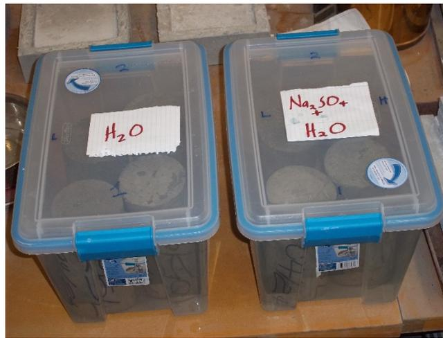
Figure 4.12 Sulfate Attack Experimental Setup
