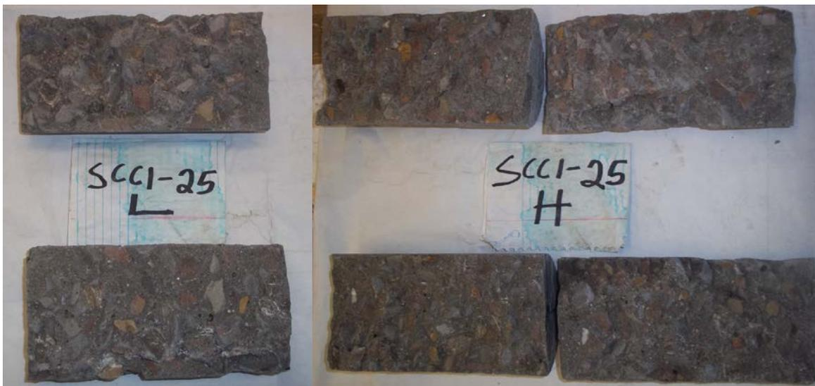
Figure 4.8 Coarse Aggregate Distribution for SCC1-25
