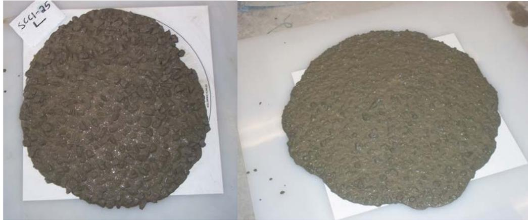
Figure 4.1 Low and High Slump Flow Diameters for SCC1-25
