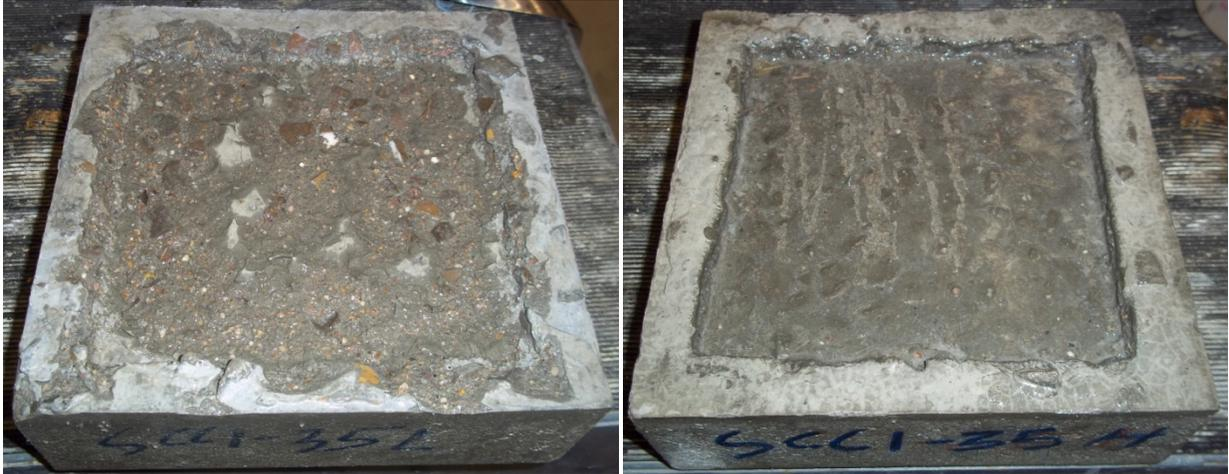
Figure 5.12 SCC1-35L (Left) and SCC1-35H (Right) after 15 freezing and thawing cycles. The specimens were inspected at specific periods to assess the impact of the NaCl solution on the respective depressed surfaces. The impacts of the brine solution on the surface were visually rated with respect to ASTM C672 surface ratings.
