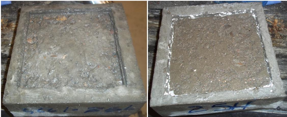
Figure 5.11 SCC1-25L (Left) and SCC1-25H (Right) after 15 freezing and thawing cycles
